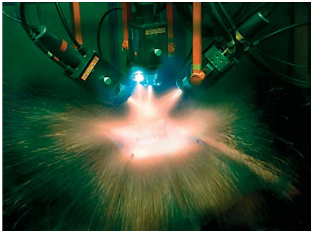
Fig. 2 Spray forming process in operation
