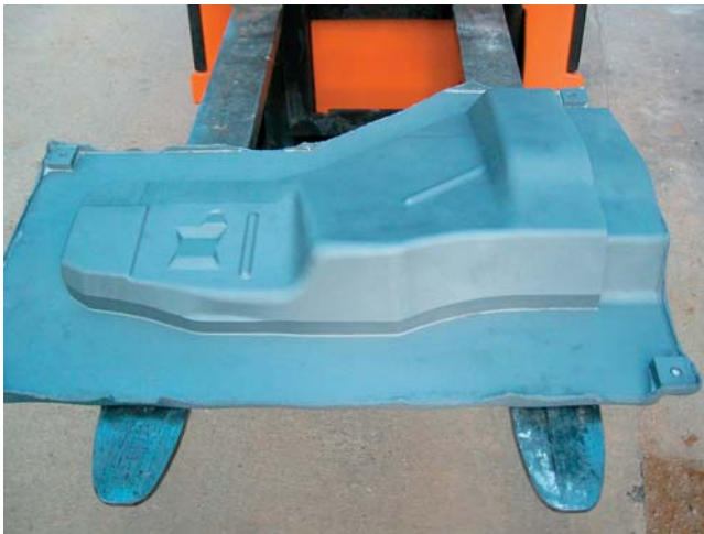
Fig. 12 A 800 by 600 mm spray formed steel shell for press tool applications, currently under assessment in volume production
