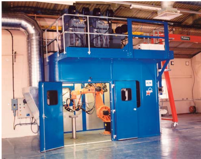
Fig. 1 Spray cell at Oxford University featuring four electric arc spray guns and a six-axis robot
